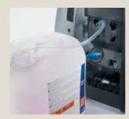
The integrated injector-doser and suction hose make application of detergent quick and simple.
